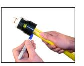
7 If using ID chamfer tool with gauge, check for proper chamfer by inserting pipe on gauge up to the o ring. With proper chamfer, o ring will begin to enter pipe.
